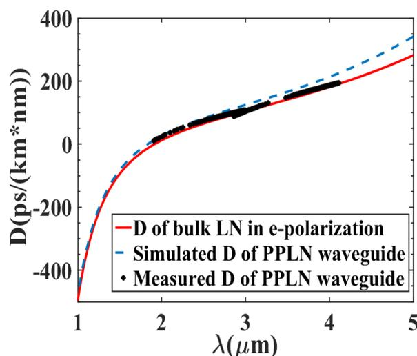
Fig.3: Measured dispersion relation and simulated group velocity dispersion
