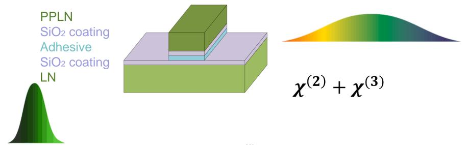
Fig.1: SCG in quadratic  $\chi^{(2)}$  nonlinear waveguides
