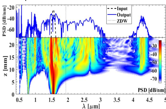
Fig.4: Numerical simulation of spectrum broadening in a 23 mm long, 26  $\mu\text{m}$  pitched PPLN waveguide pumped by 125 fs laser with peak power of 10.4 kW at 1550 nm.
