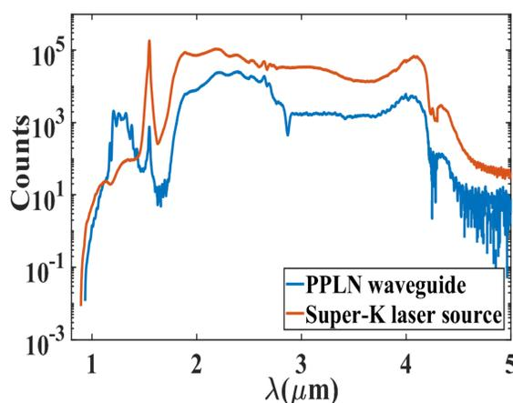
Fig.2: Measured transmission of the waveguide.
