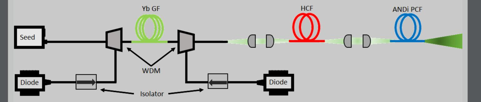
Figure: Schematic of the optical setup composed by a femtosecond seed, an amplifier, a compressor and a nonlinear stage
