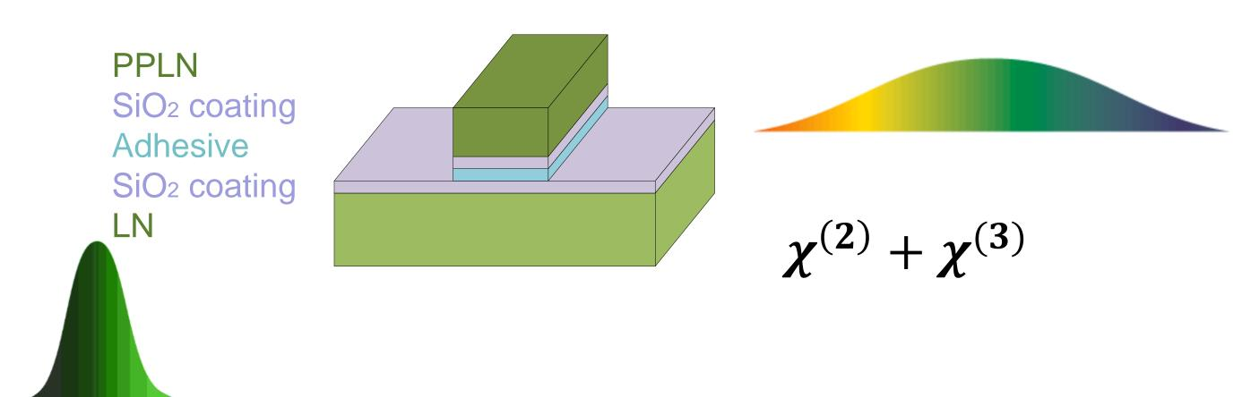
Fig.1: SCG in quadratic  $\chi^{(2)}$  nonlinear waveguides
