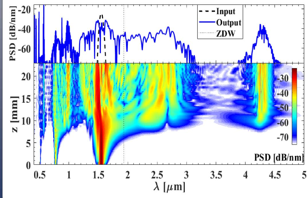
Fig.4: Numerical simulation of spectrum broadening in a 23 mm long, 26 µm pitched PPLN waveguide pumped by 125 fs laser with peak power of 10.4 kW at 1550 nm.
