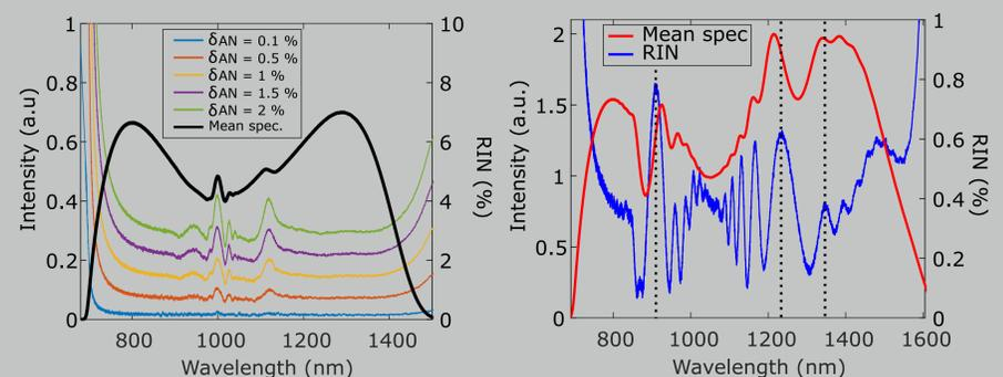
Figure: RIN profile for different amplitude noise values (color curves) and mean spectrum of an ensemble of 20 pulses (bold black curve) after 1 m of fiber with 100 kW peak power, 50 fs pulse duration at 1054 nm for an amplitude noise value of 0.5 %. RIN profile (blue line) and mean spectrum (red line) of an ensemble of 20 pulses after 10 cm of fiber with 100 kW peak power, 50 fs pulse duration at 1054 nm for an amplitude noise value of 0.5 %.
