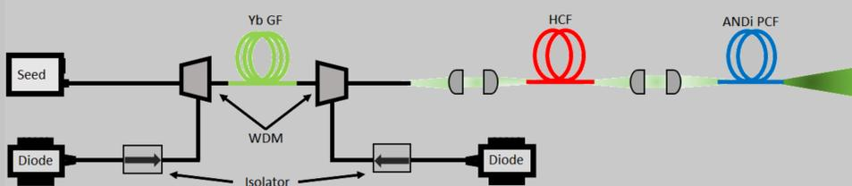
Figure: Schematic of the optical setup composed by a femtosecond seed, an amplifier, a compressor and a nonlinear stage
