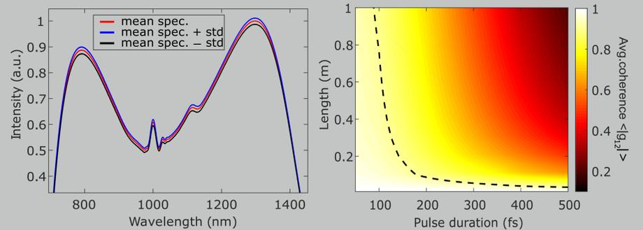
Figure: Numerical supercontinuum spectra after 1 m of ANDi fiber showing fluctuation in spectral power and shape for 0.5 % amplitude noise and a pulse duration standard deviation of 0.4 fs. The simulation uses an average pulse duration of 50 fs and a peak power of 100 kW at 1054 nm. Average spectral coherence of SC pulse generated with 100 kW peak power pump pulses as a function of pump pulse duration and propagation distance including an amplitude noise value of 0.3 %.
